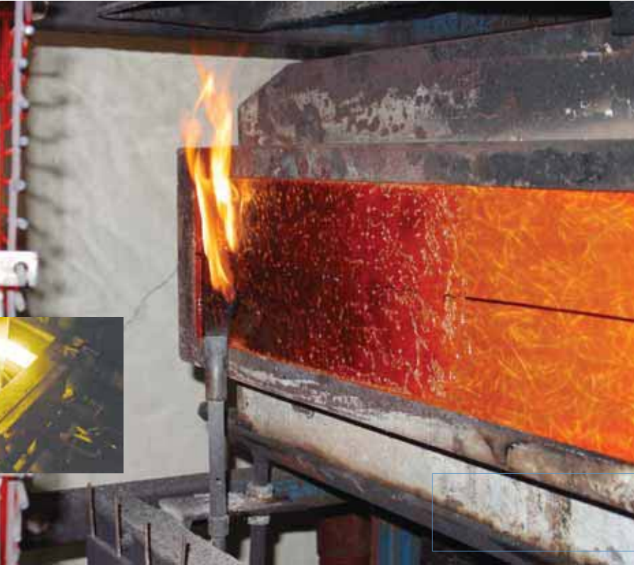
IMO A.653 (16) Fire Hazard Test conducted at CSIRO
